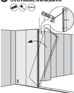
Secure the last panel to the T-profile and secure all panels with (27cm) anchoring straps in the upper groove.
