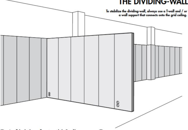
Install the dividing-wall starting with the T-profile.
